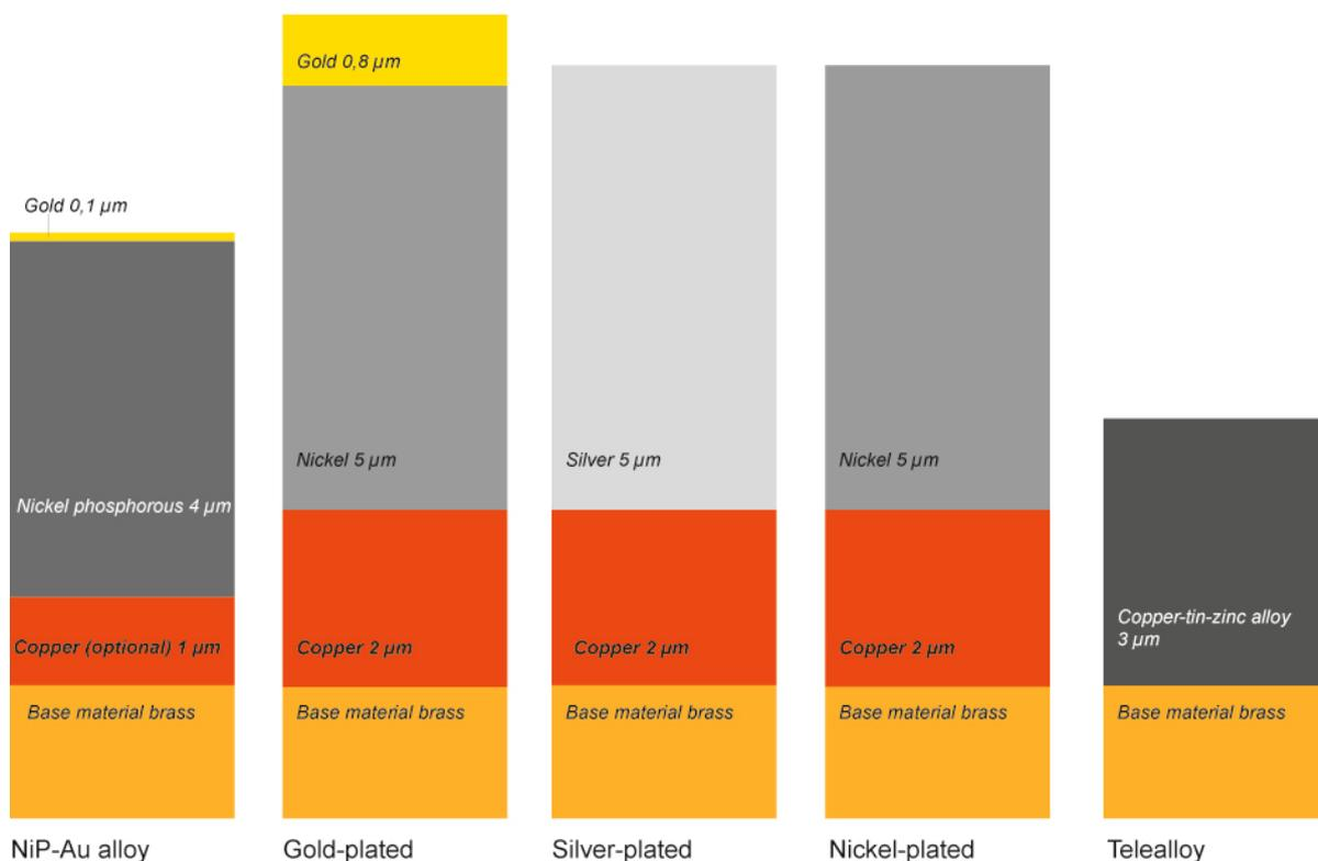
*Frequently used materials for coaxial HF connectors*
