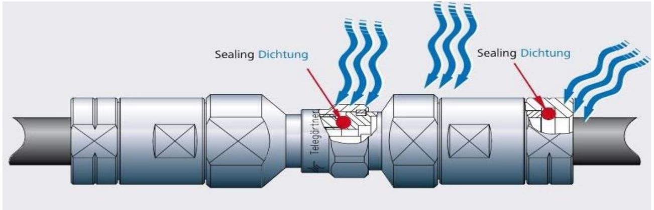
Figure 8: Transverse tightness of the entire plug system
