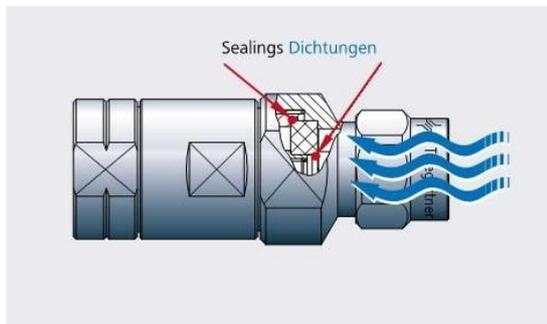
Figure 6: Longitudinal tightness in unplugged state
