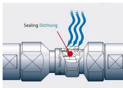
Figure 7: Transverse tightness in the connection face
