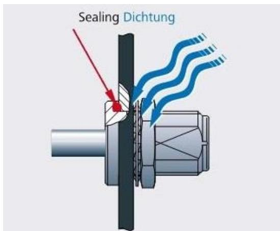
Figure 9: Installation tightness
