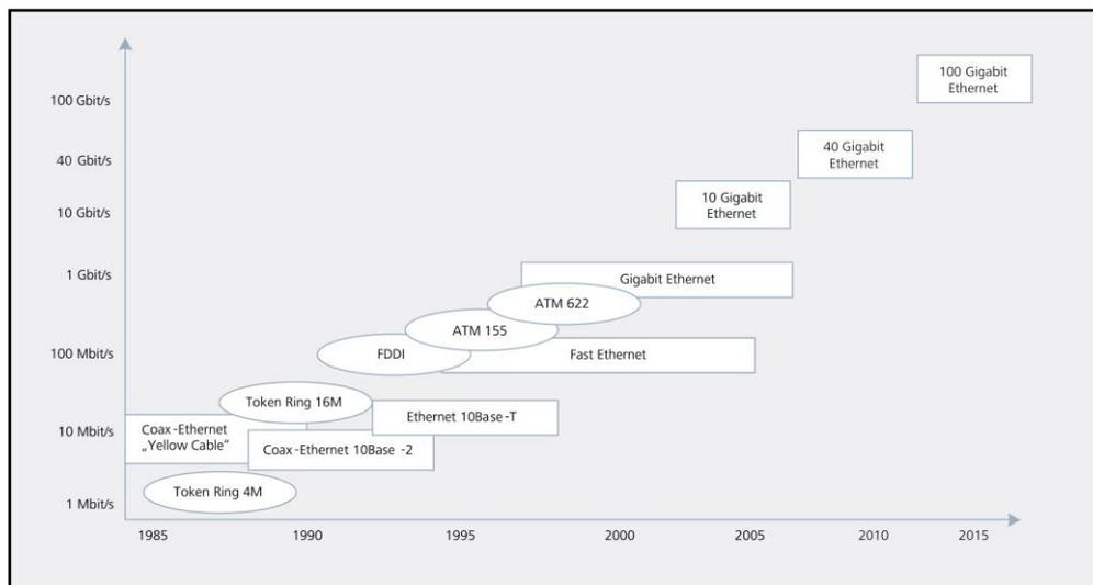
**Development of LAN technology:** Ethernet has become established as the main LAN technology. Fast Ethernet and Gigabit Ethernet are most commonly used, with 100 Mbit/s and 1 Gbit/s respectively. 10 Gigabit Ethernet with 10 Gbit/s is used for very fast connections and is supplemented by 40 and 100 Gigabit Ethernet.
