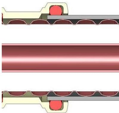
Figure 2: Inherent pressure seal
